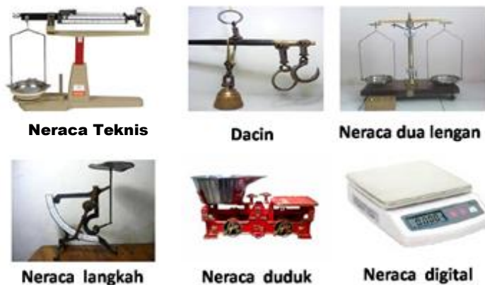
Gambar 2. 5 Macam alat ukur massa
