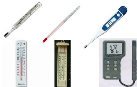
Gambar 2.8 Macam alat ukur suhu
